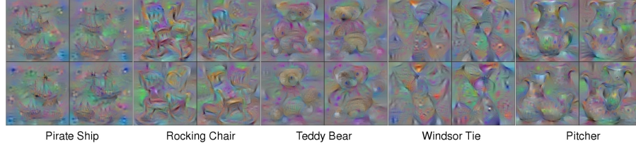
Figure 2.11: Feature maps produced by later convolution layers. Yosinski et al. [26].
