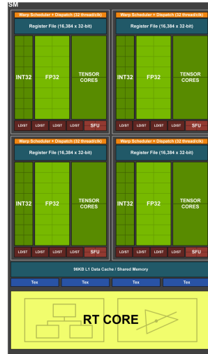
Figure 2.3: Structure of the Turing streaming multiprocessor.
